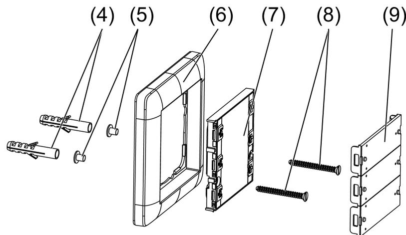
Figure 16: Screw mounting
