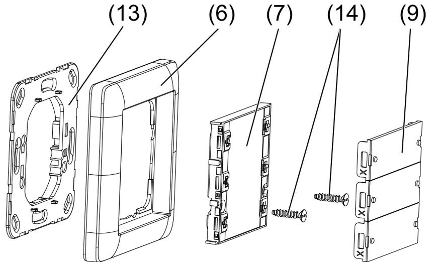
Figure 18: Installation in appliance box
